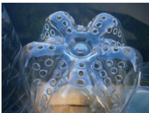
Above: Holes in bottom of main chamber
